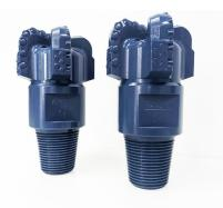
It is an ideal drill bit to use in sandstones limestones and in the transition from heavily weathered crystalline rocks into the consolidated fresh underlying rock to drill pockets to set surface casing to allow drilling to switch to compressed air and DTH down The Hole hammer and percussive button bit.
