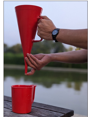
Marsh Funnel & Jug (to measure mud viscosity)
