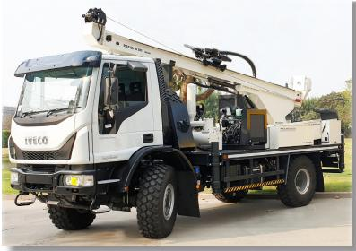
For Down-the-hole-hammer and mud rotary drilling up to 300 m depth 150-245 mm (6"-10") diameter – according to tool selection.
