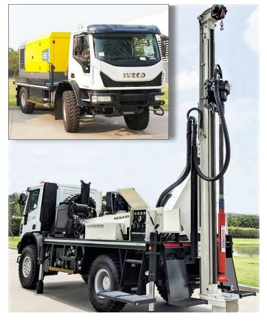
PAT-Drill 501 4x4 mounted on IVECO 4x4 off-road truck 15,000 GVW. (Available left or right steering)
