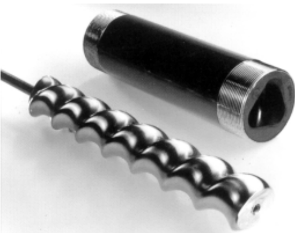
Figure 2.1 Progressive cavity pumping method
