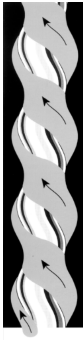
Figure 2.1 Progressive cavity pumping method
