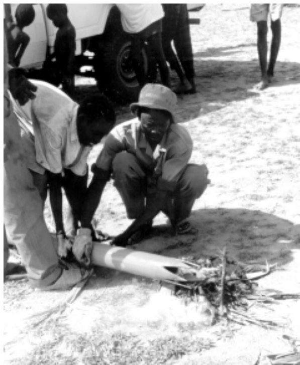
Figure 7.2 Heating up pipe end to form points
