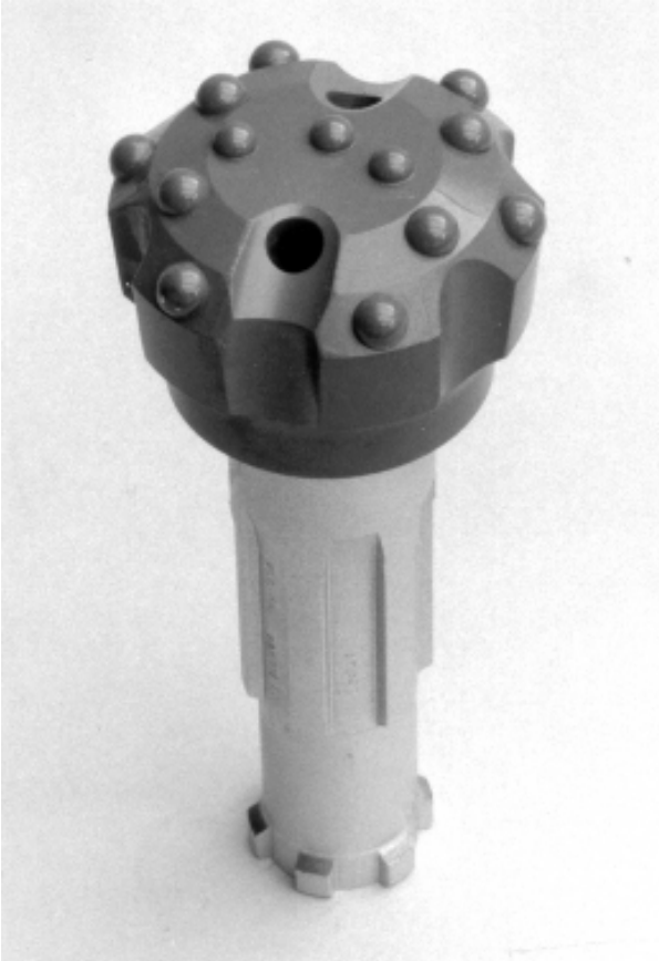
Figure 1.2 Down-the-hole-hammer tungsten button drill bit
