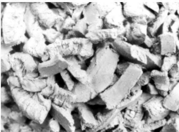
Figure 2.9 Individual clay cuttings washed to the surface
