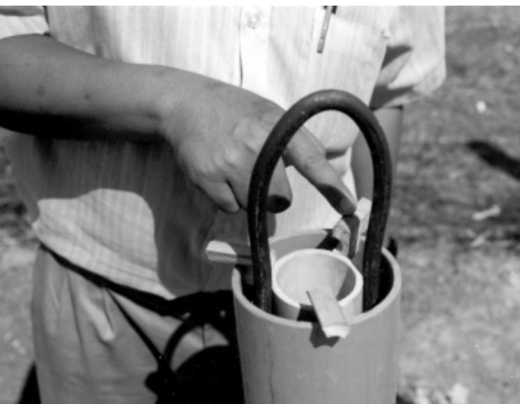
Figure 7.1 Construction of hollow weighted dummy – ready for filling for weight with cement
