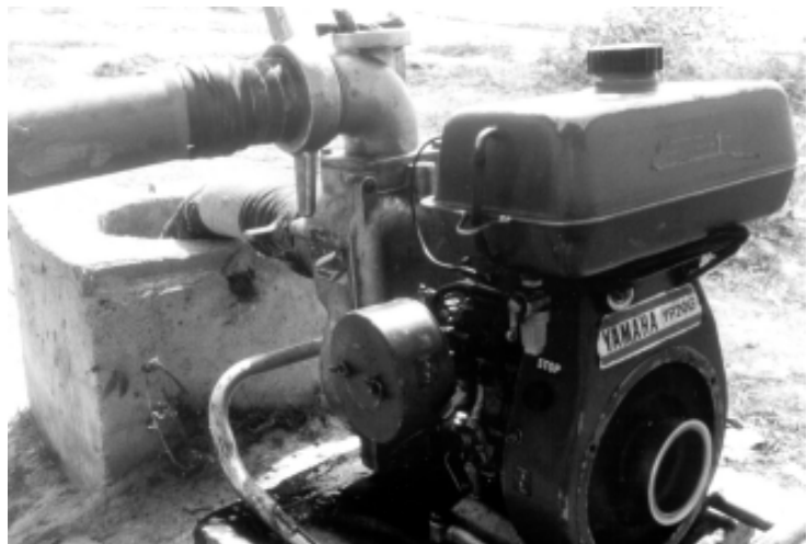
Figure 6.6 Centrifugal pump drawing water from a 100mm (4") tubewell
