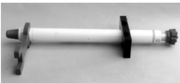
Figure 3.3 Down-the-hole hammer – with stripping clamp and spanner
