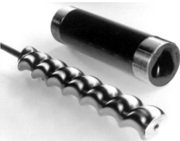
Figure 2.1 Progressive cavity pumping method
