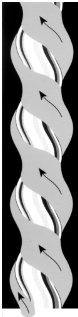
Figure 2.1 Progressive cavity pumping method
