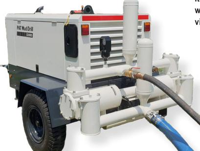
It can be used with bentonite, polymer and weighted drill mud additives through various viscosity and densities
