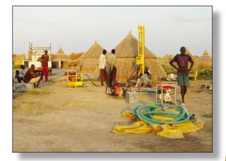
Rig is powered by a stand alone power pack with a heavy duty Diesel engine or lightweight Petrol engine option.
